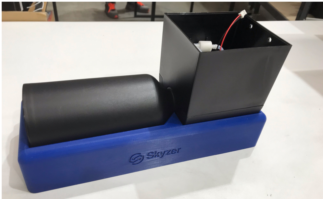
Photos: Customised jig used to maintain components at an incline during assembly.
